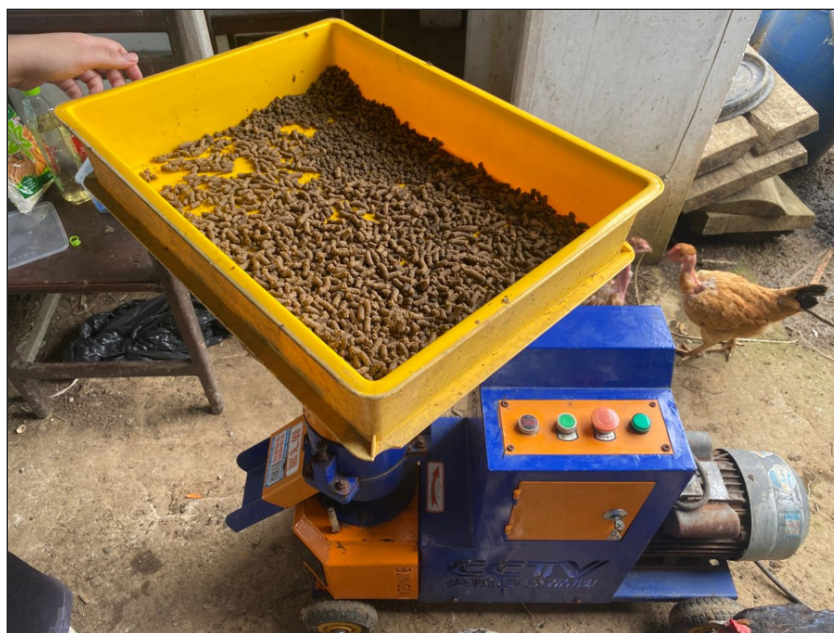
Figure 1. Pelletizer machine producing uniform feed pellets
